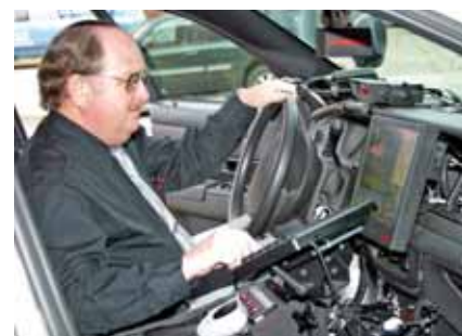
The monitor mounts directly to the dash with Hub-Data911's Mobile Digital Computer (MDC).
