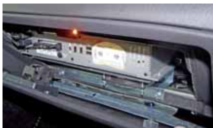
Hub-Data911's Central Processing Unit (CPU) can be popped out of the glove compartment if necessary.
